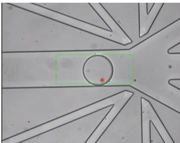
**Fig. 1:** Example of cell detection (red square) in the region of interest (green rectangle) before a droplet sorting process. Diameter of droplet is  $80\mu\text{m}$ .
