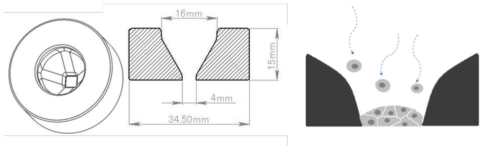
**Figure 1.** Dish holder for cell sedimentation.
