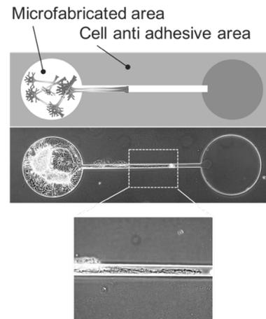
Figure 2. Combination technique of 2.5D and agarose microfabrication technique
