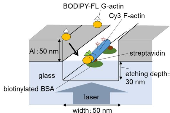
Fig. 1 Experimental setting with linear zero-mode waveguides
