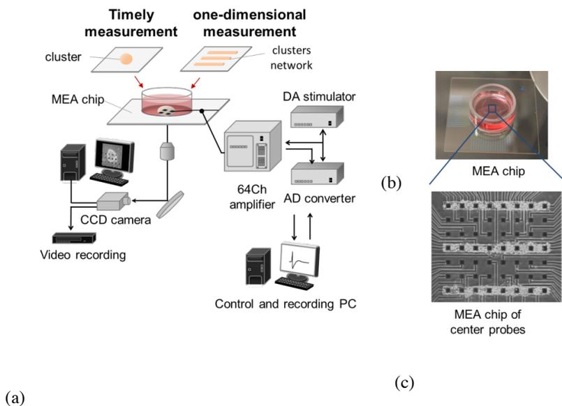
**Figure 1.** (a) Schematic of an on-chip multi electrode array system. (b) Schematic of a MEA chip. (c) Clusters of cardiac muscle cells which were lined-up on a surface of MEA chip.
