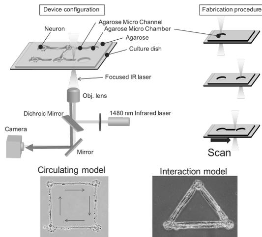
Figure 1. Agarose microfabrication technique
