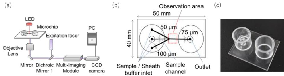
**Figure 1. Overview of the on-chip multi-imaging cell analysis flowcytometry.** (a) Schematic image. (b) Design of the microchip. (c) Image of the microchip.
