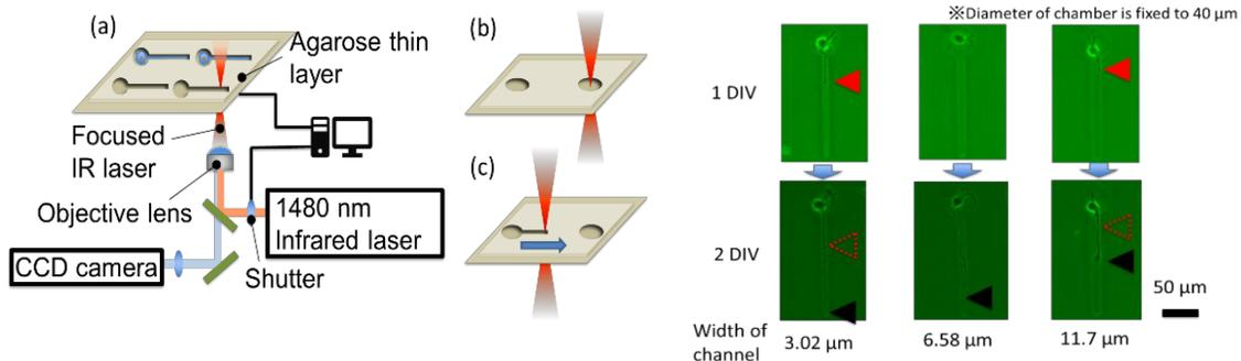
**Fig. 1.** Design (a) and procedures (b, c) of *in situ* photothermal microfabrication method. Microstructures of agarose are fabricated by spot heating of IR laser during cultivation.
