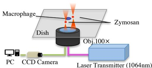
**Fig.2. Two-way optical tweezers and observation assay.** We caught a zymosan by optical tweezers, and carried on a macrophage.
